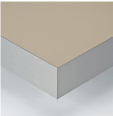
AP10-...-08 Front edge with laminate edging. The appearance of a worktop 95 mm thick is achieved via the doubled frame construction. The recess height is reduced accordingly.
