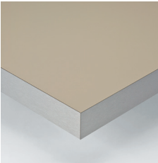
AP6-...-08 Front edge with laminate edging. The appearance of a worktop 57 mm thick is achieved via the doubled frame construction. The recess height is reduced accordingly.
